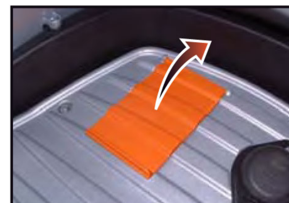
1. Lift out the cover to disconnect the plugs.
