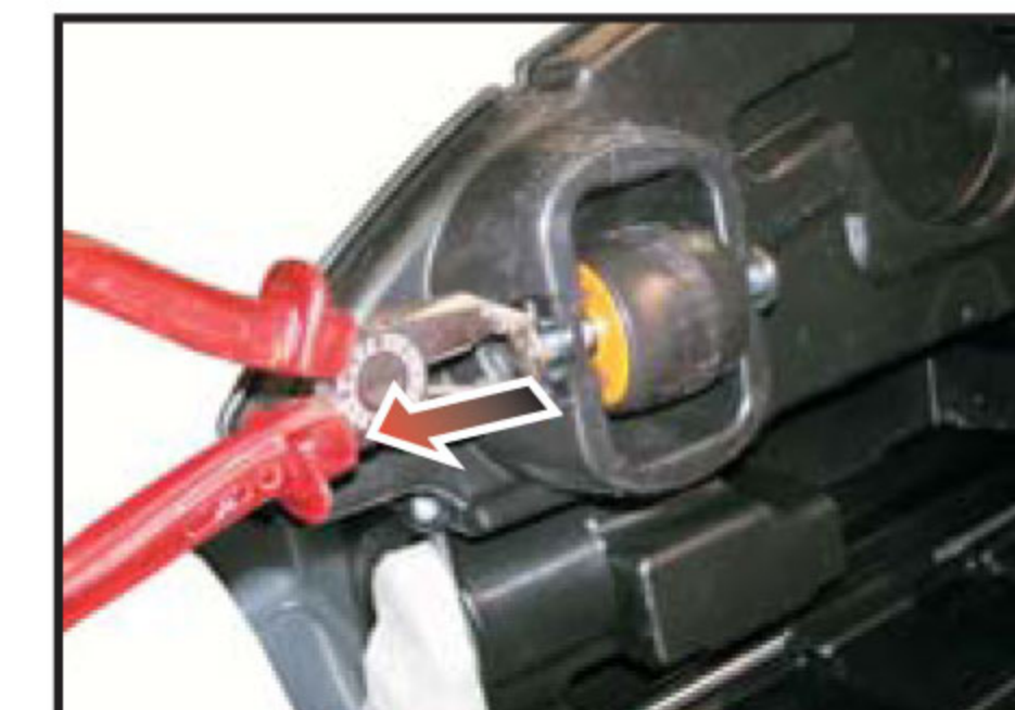
1. Remove the aranlock from the axle of the small wheel.
