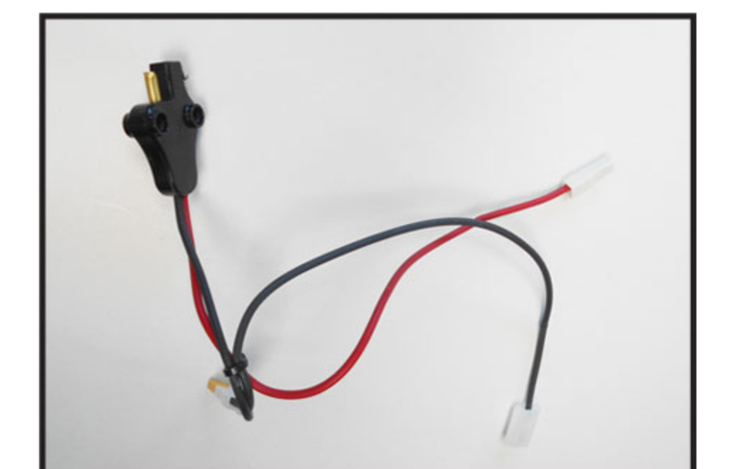
6. Replace the wires and re-assemble in reverse order. Note: Pay attention to connecting the wires to the proper polarity marked on the battery.
