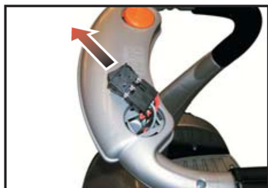
3. Disconnect the button switch and replace it with a new one. Re-assemble in reverse order.
