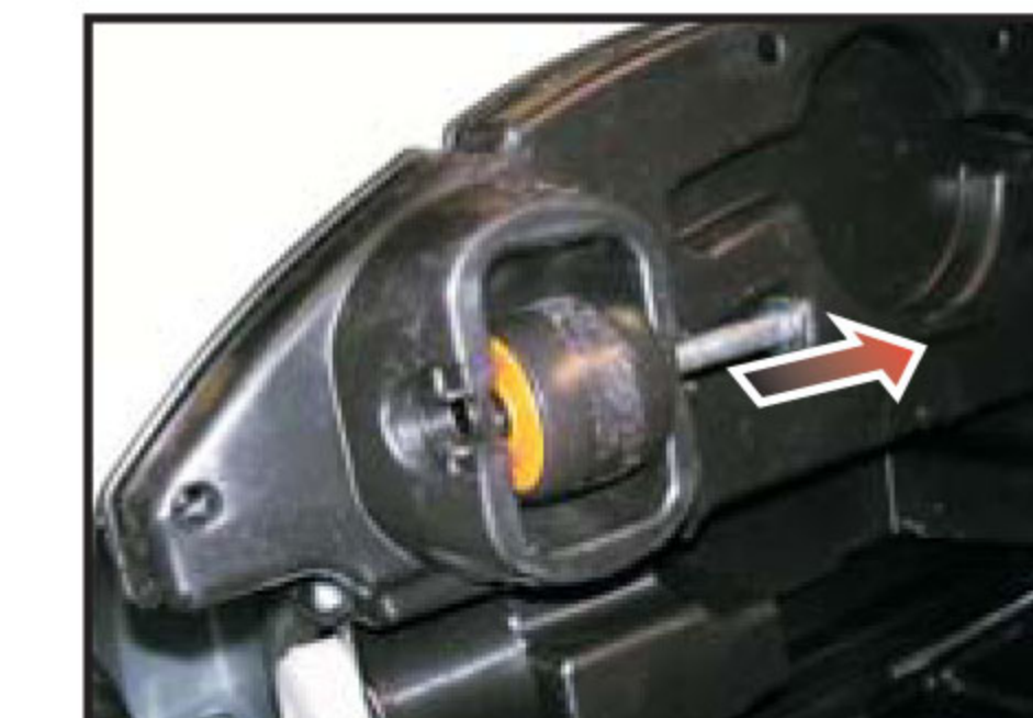
2. Remove the axle from the wheel.
