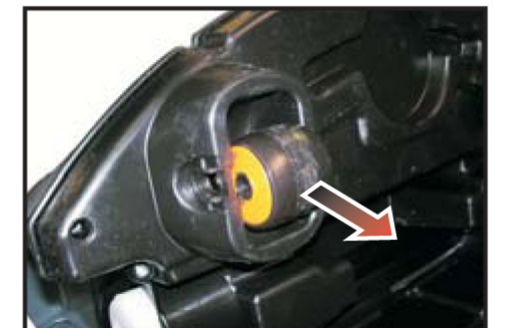
3. Remove the wheel which does not work, replace it with a new one. Re-assemble in the reverse order.
