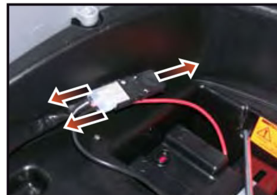
2. Disconnect the circuit breaker to replace it with a new one. Re-assemble in reverse order.
