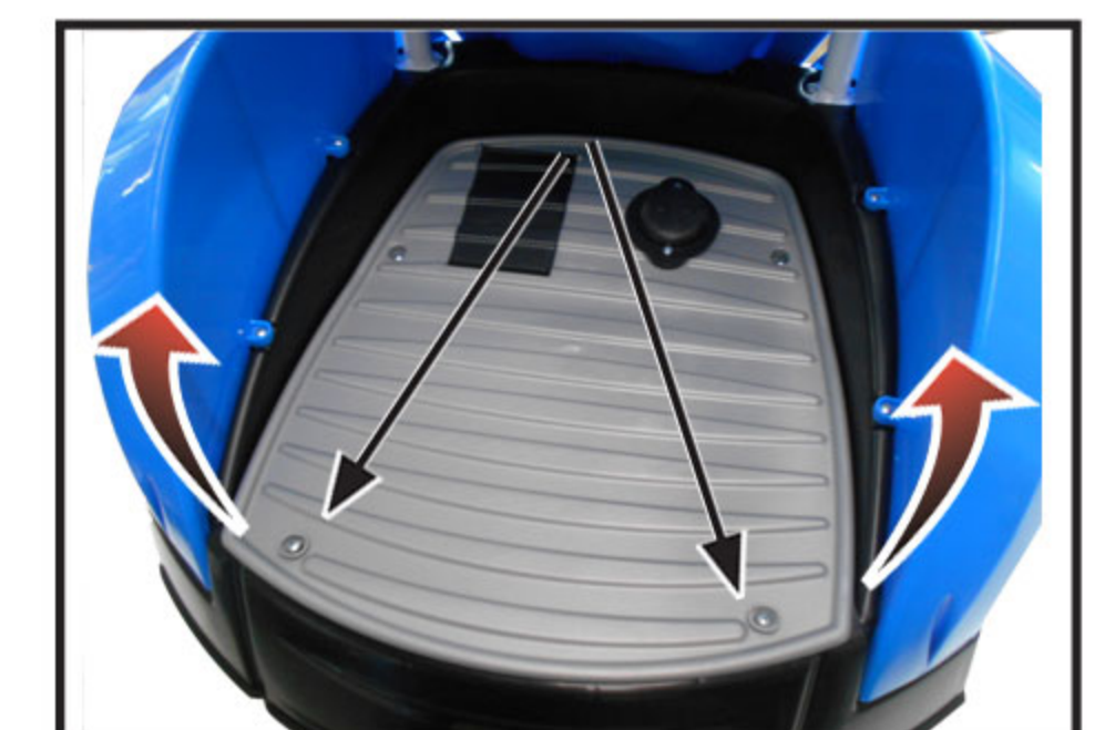
3. Unscrew the 4 screws from the dareway base.
