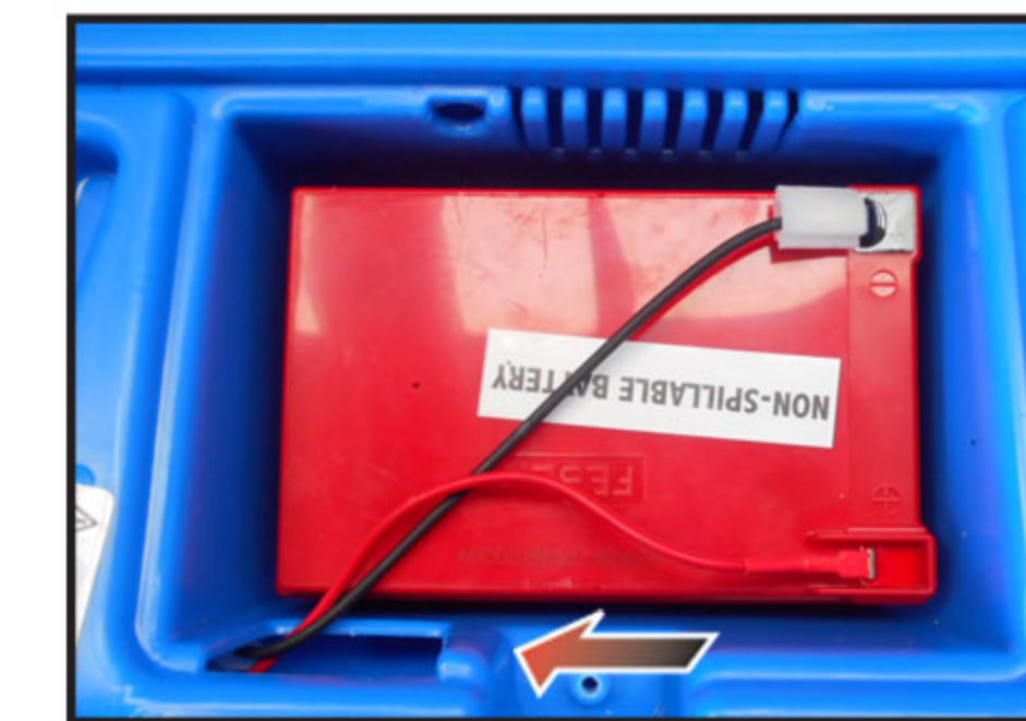
5. Disconnect the wires from the battery.
