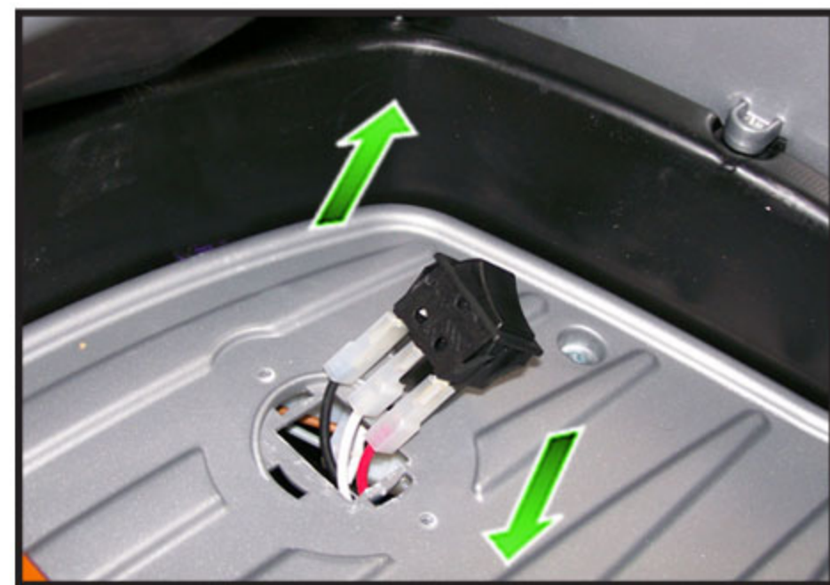
4. Disconnect the button switch and replace it with a new one. Re-assemble in reverse order.
