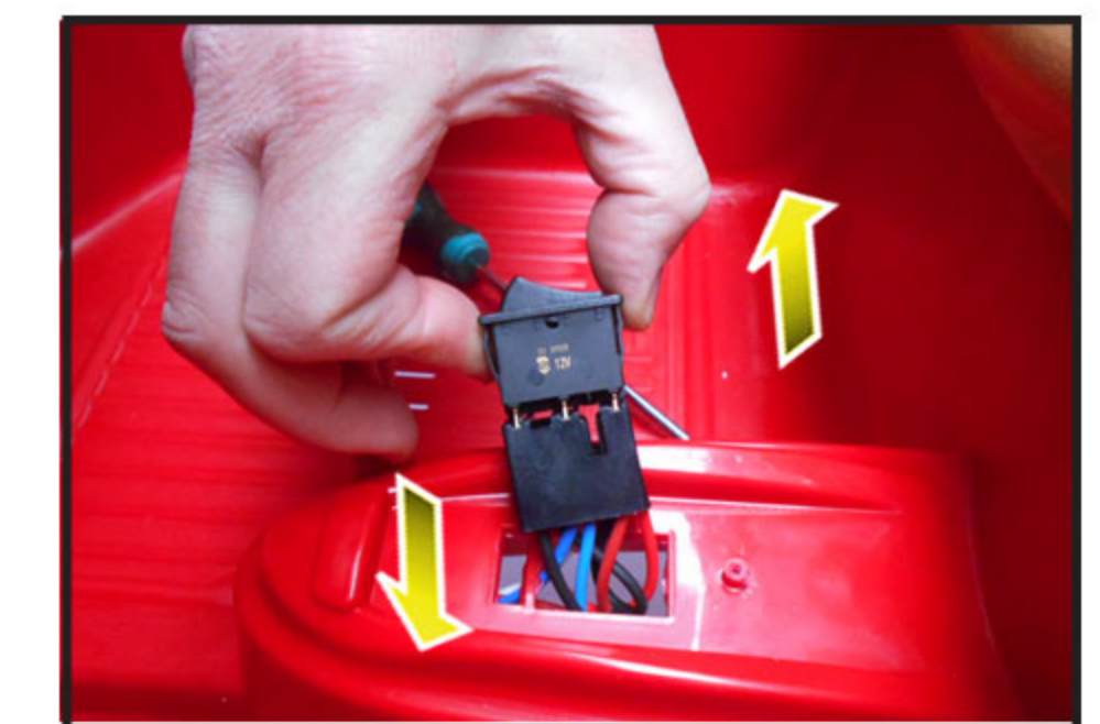
3. Disconnect the switch and replace it with a new one. Re-assemble in reverse order. Pay attention to connecting the button switch and the accelerator in the correct way.
