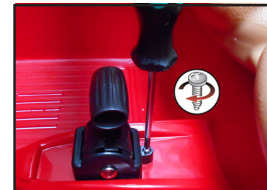
1. Unscrew the gear stick.
