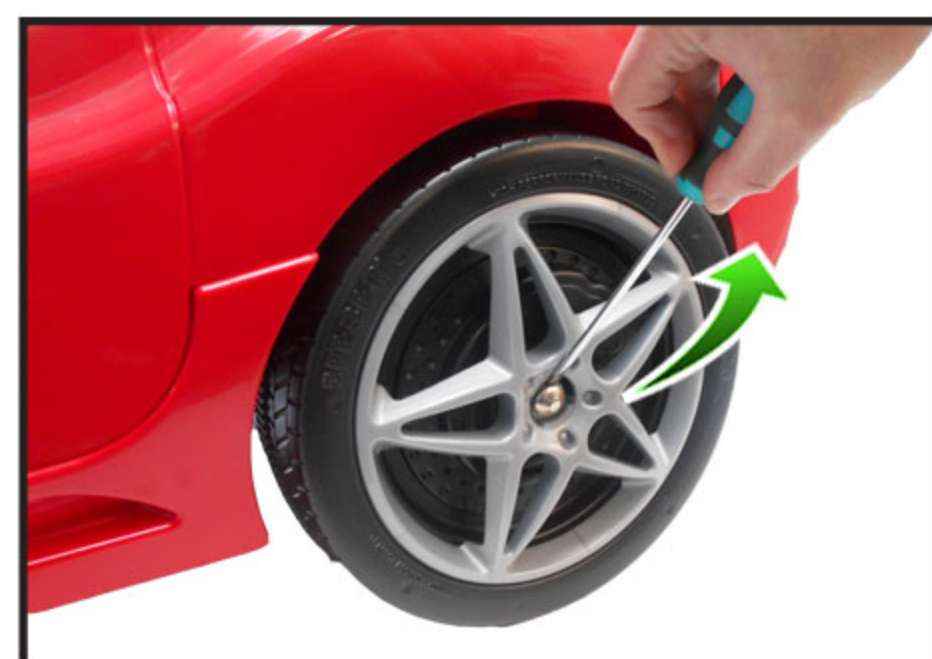
2. Remove the aranlock and the hubcap.
