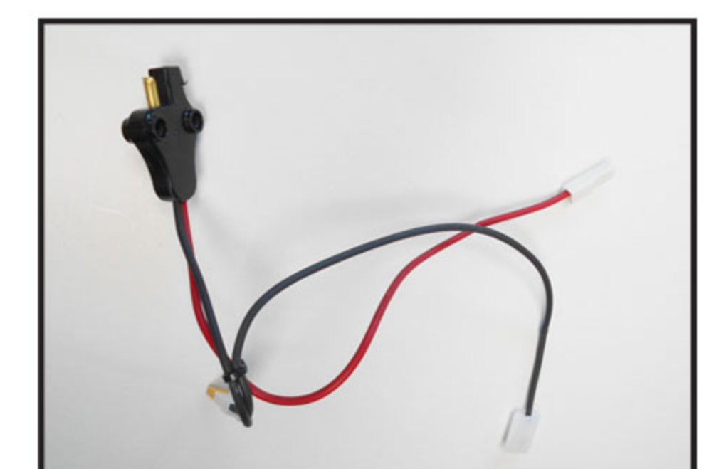
6. Replace the wires and re-assemble in reverse order. Note: Pay attention to connecting the wires to the proper polarity marked on the battery.
