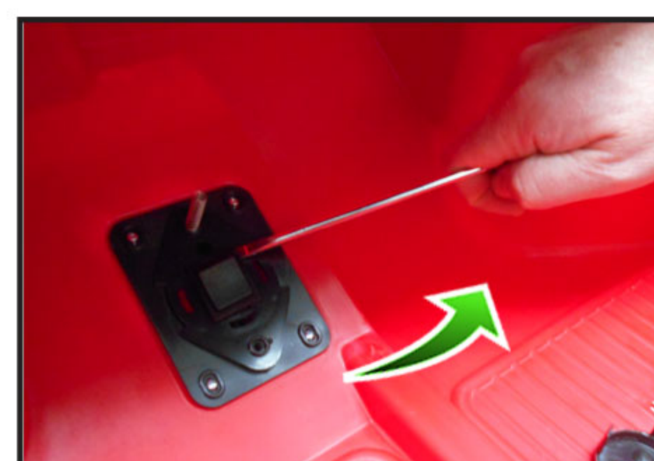
3. Remove the button switch.
