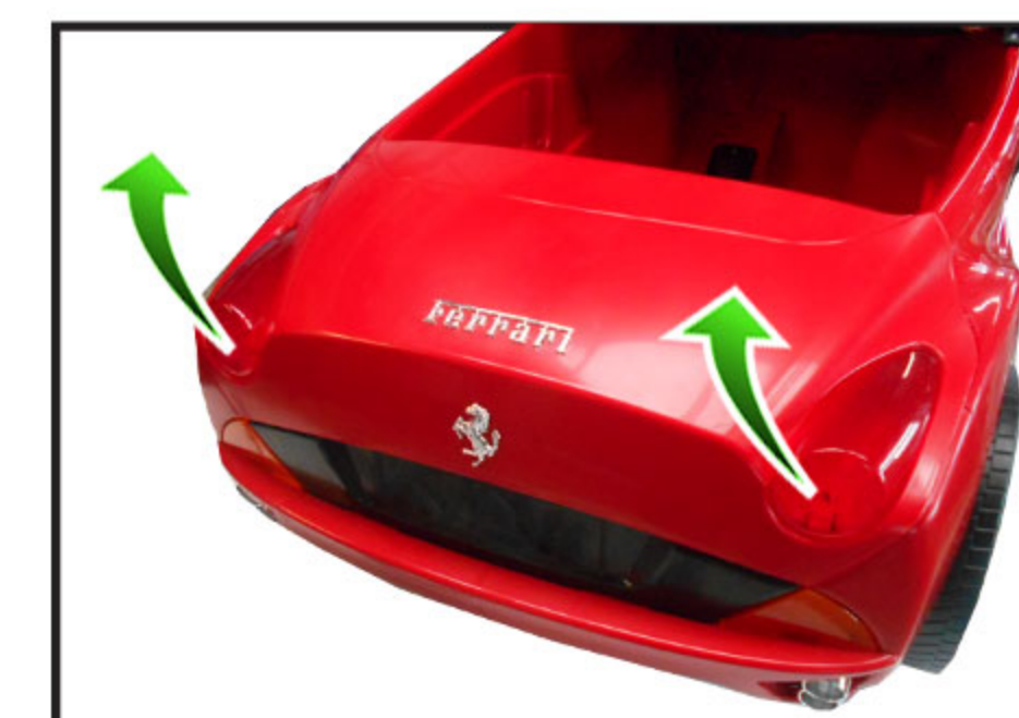
2. Remove the turn signals to find the screws.
