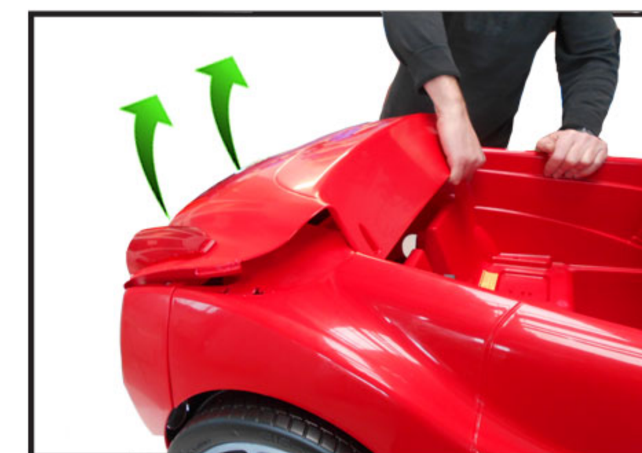
4. Remove the back side of the car.
