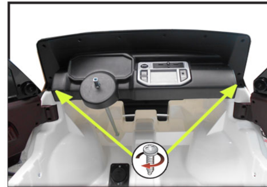
3. Unscrew the back side of the windshield.
