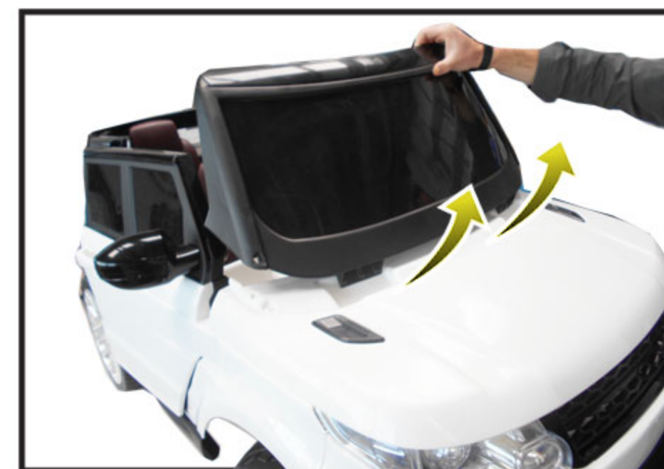
6. Remove the windshield and replace with a new one. Re-assemble in reverse order.
