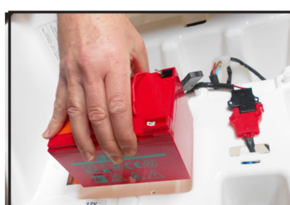
6. Remove the battery and replace with a new one. Re-assemble in reverse order and pay attention to connecting the wires to the proper polarity.
