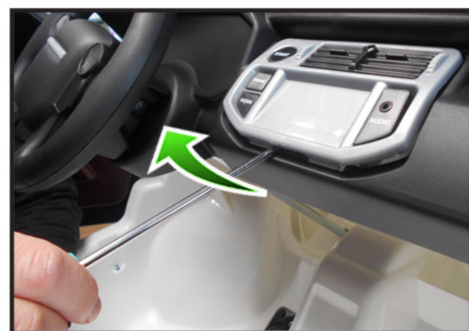
1. Remove the sound system from the car.
