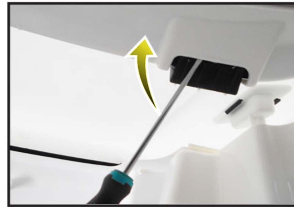
5. Release the windshield pushing the flaps out.
