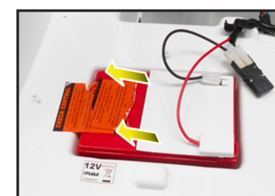
5. Disconnect the wires from the battery.
