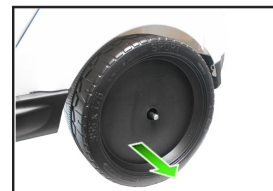
4. Remove the wheel and replace with a new one. Re-assemble in reverse order.
