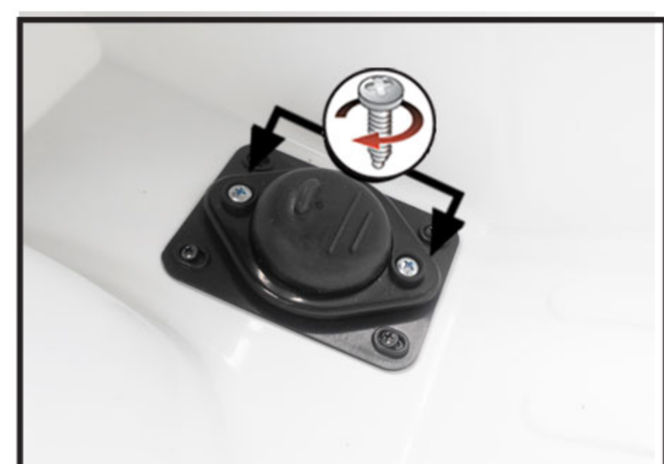
1. Unscrew the 2 screws and remove the accelerator rubber.
