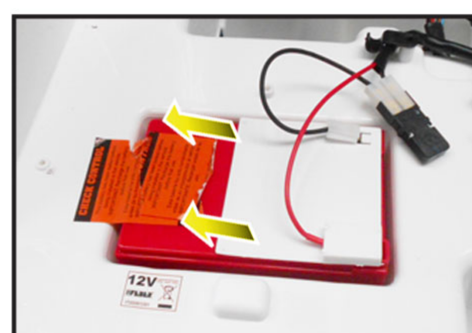
5. Disconnect the wires from the battery.
