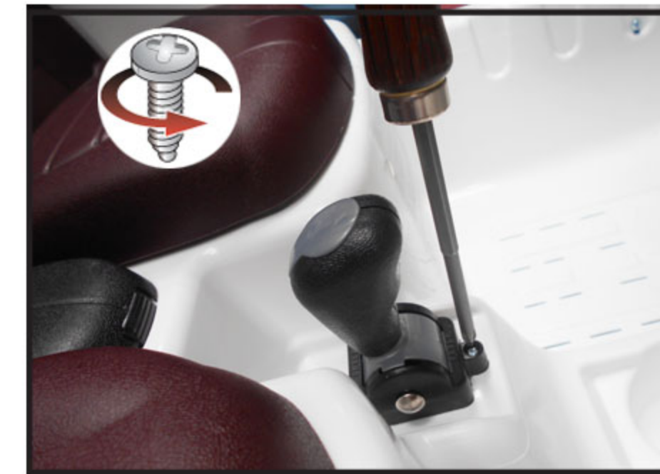
1. Unscrew the gear stick.
