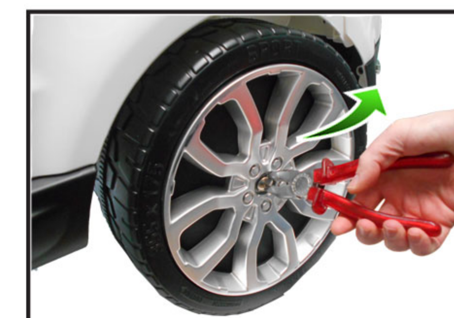
2. Remove the aranlock and the washer.
