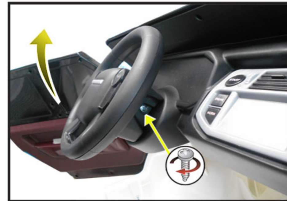
2. Unscrew the steering wheel.
