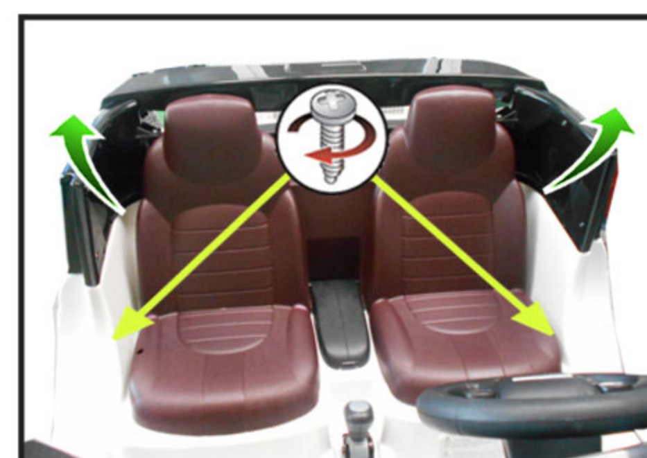
3. Unscrew the front side of the seats and remove them.
