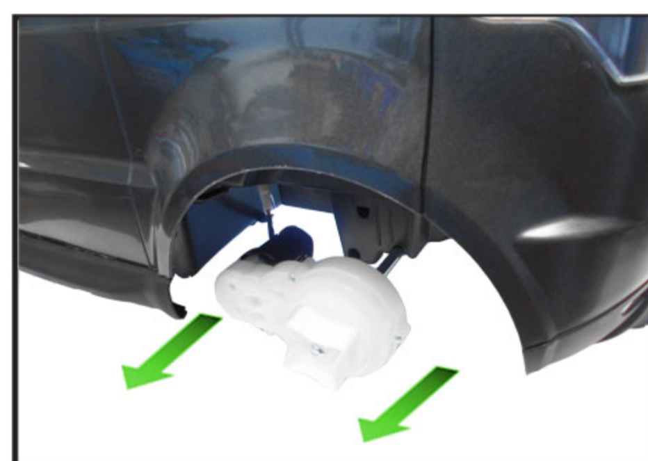
5. Remove the mechanism.
