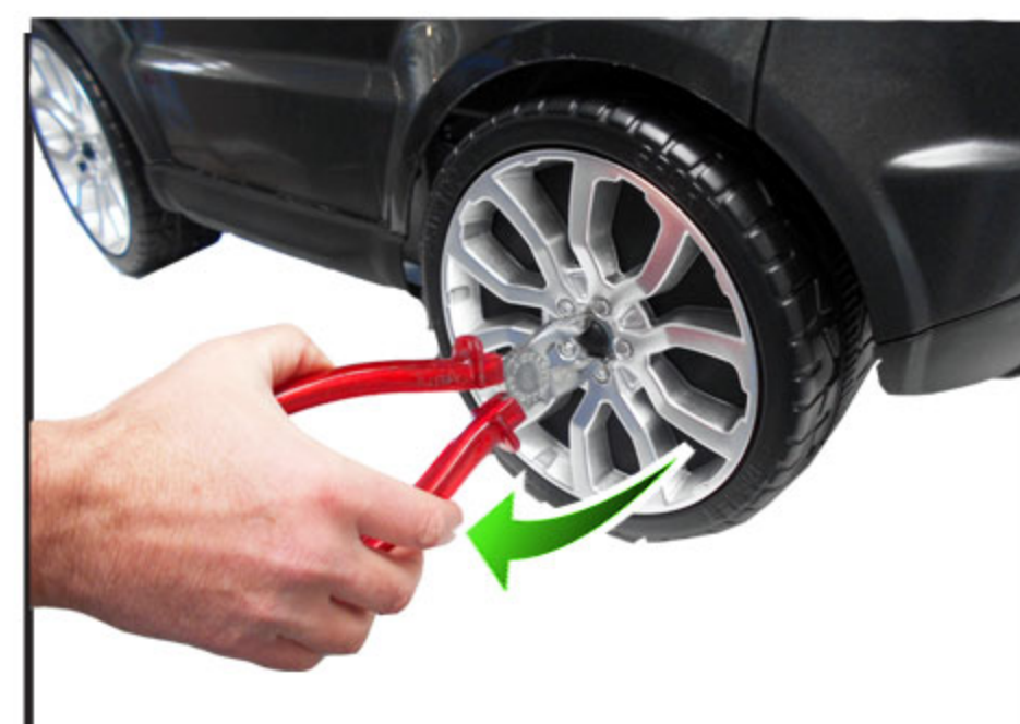
1. Remove the axle lock and the washer.
