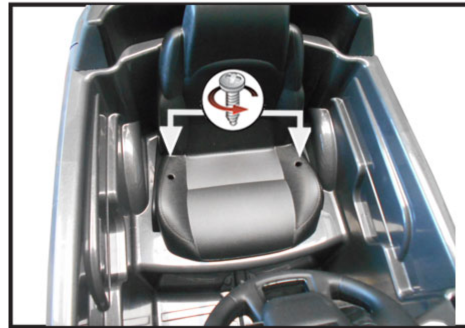
1. Unscrew the 2 screws from the seat.
