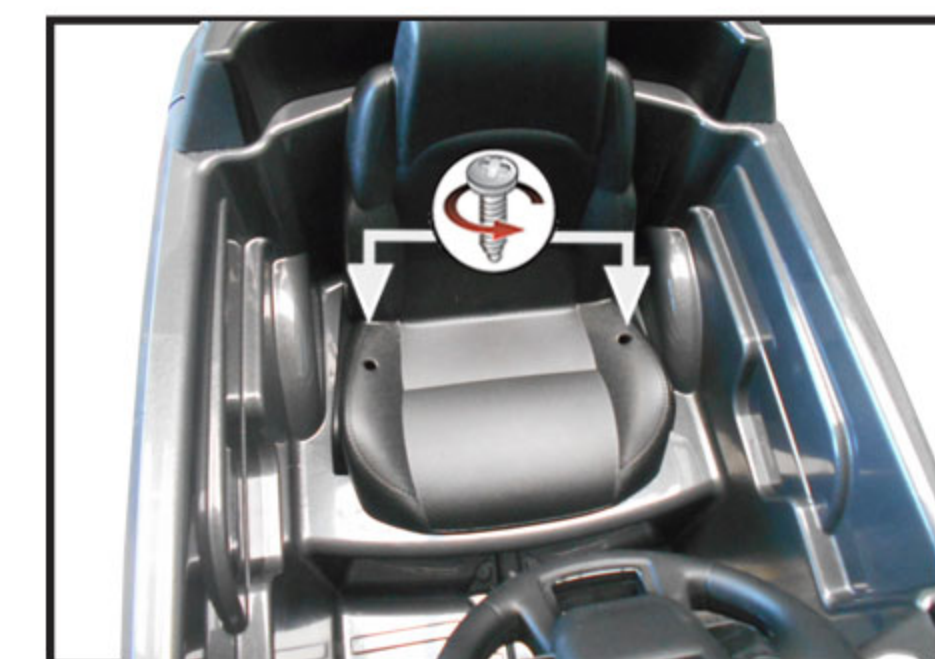
1. Unscrew the 2 screws from the seat.
