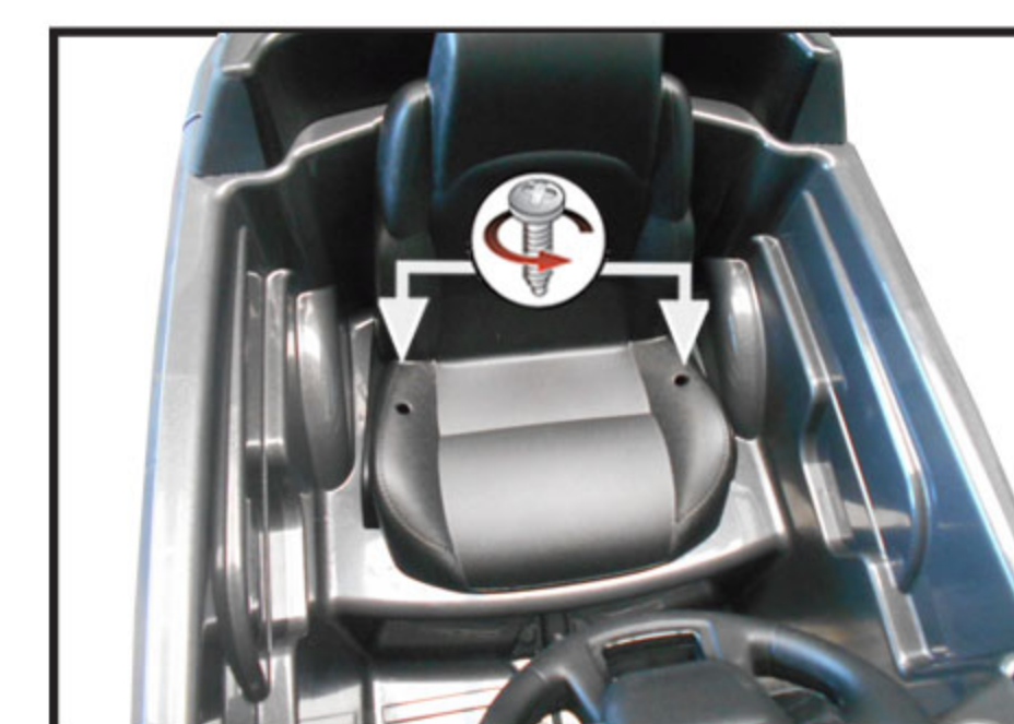
1. Unscrew the 2 screws from the seat.
