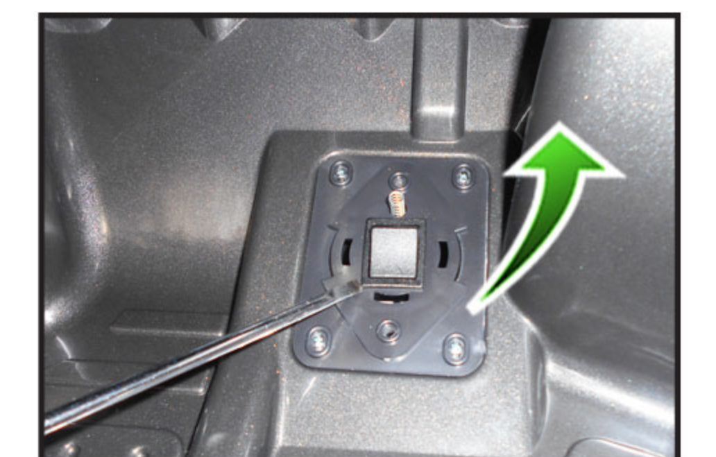
3. Remove the accelerator button.
