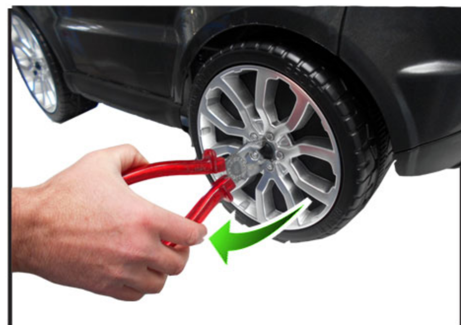
1. Remove the axle lock and the washer.
