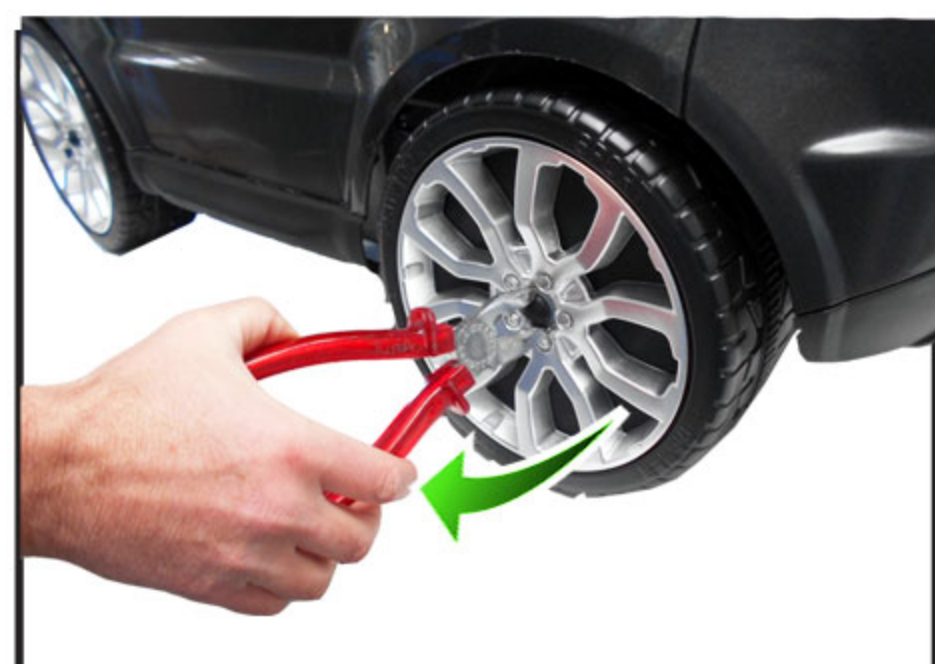
1. Remove the axle lock and the washer.
