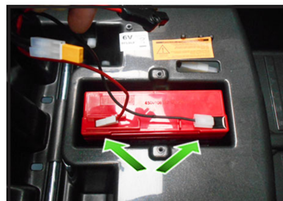
7. Disconnect the wires from the battery.
