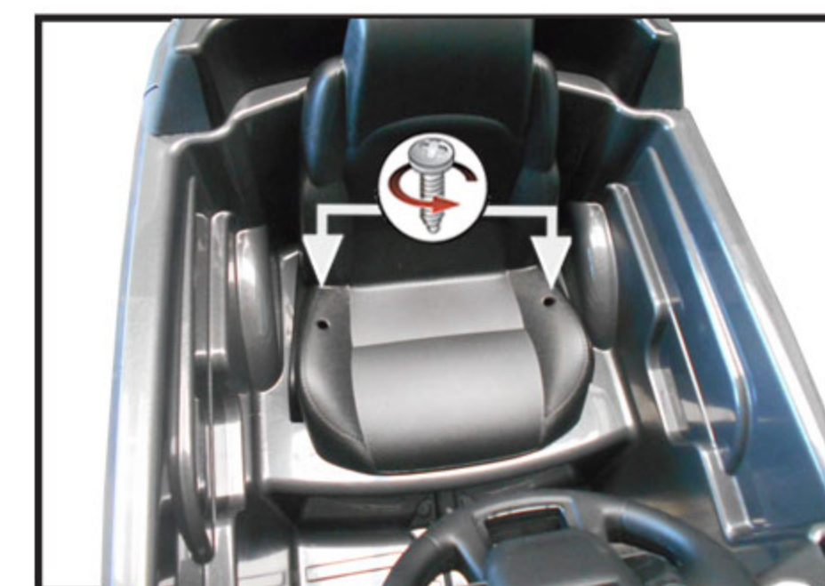
1. Unscrew the 2 screws from the seat.
