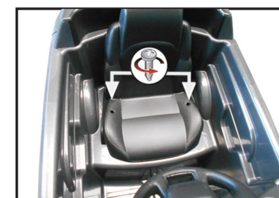
1. Unscrew the 2 screws from the seat.
